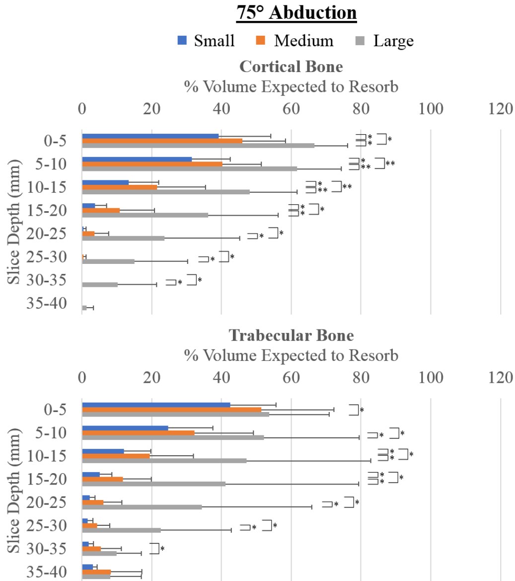
Figure 2-14: Changes in Percent Volume of Bone Expected to when Implant Girth was Increased at 75° Abduction
